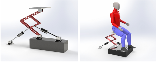
Fig. 3. Proposed gravity balanced robotic architecture
